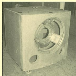
Prototype woofer enclosure, preliminary mechanical and acoustic testing
