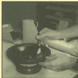
Doping the cone of the first prototype 10" unit
